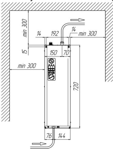
Figure 3 Example of mounting the boiler on the wall
